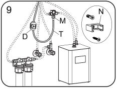
9. Tidy up all hoses, so they don't get tangled up. Please leave enough space for the pull-down hose (T) with counterweight (D) to move up and down without interference to ensure the pull down function. The wall mount can be screwed to the wall, and three-way quick connector can be attached to the wall mount. See Fig.9.
