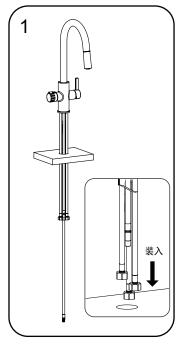
1. Taking the faucet from packaging box and place six hoses into mounting hole one by one. See Fig.1
