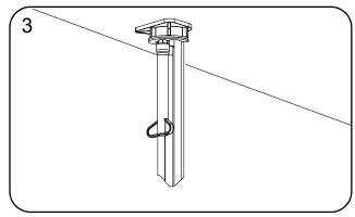
3. Adjusting the faucet at correct direction,and tighten the mounting nut (H) with wrench (I). See Fig.3
