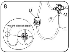
8. Attach the pull-down hose (T) (with label ⑦/white color) to the adapter at the bottom of the three-way quick connector (M). Installing the counterweight (D) on the marked position of pull-down hose. See Fig. 8
