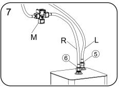
7. Connecting boiling water supply hose (L) (with label ⑤/green color) to the inlet of boiling water tank. Connecting one end of Boiled water outlet hose (R) (with label ⑥/red color) to otlet of boiling water tank, and connecting the other end of hose (R) to another adapter of three-way guick connector (M).See Fig.7
