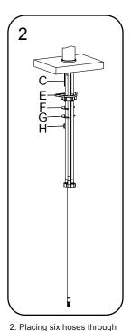
nut (H) to fix rubber washer (F) and metal wahser (G) on screw stem (C).See Fig.2
