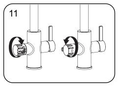
11. Sliding out the pick on the left round handle and turning the round handle clockwise at the same time, it will comes out the boiled and filtered water. And turning the round handle counter-clockwise, it will comes out the cold and filtered water.
