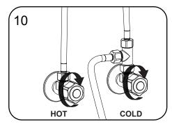
10. Turn on the water supply and check the water connections for leaks. Test system for leaks, and purge system.Run a minimum of 20 litres of water through the tank to remove any air. See Fig.10.
