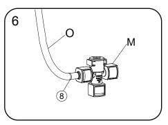
6. Connecting the three-way quick connector (M) to outlet hose (O) (with label ®/white color). See Fig.6
